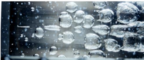
Figure 12 Bubble cavitation on a foil evaluated in the cavitation tunnel
