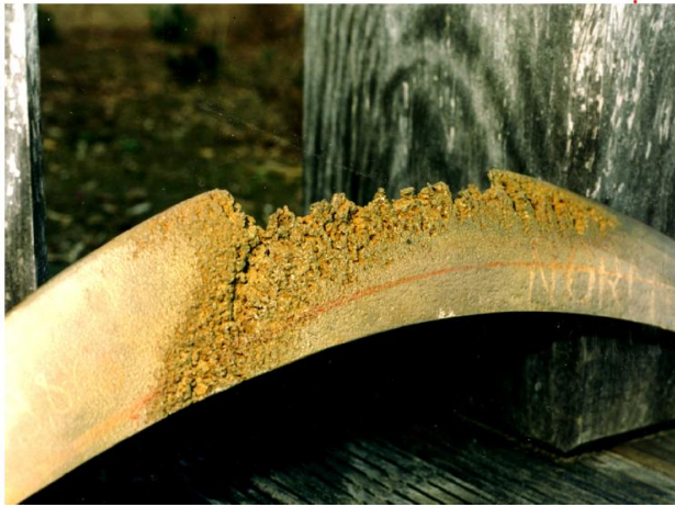
Figure 23 Erosion due to cavitation Full scale
